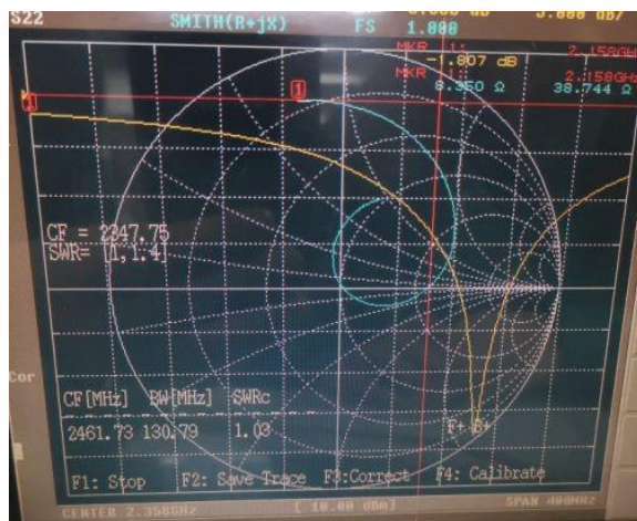
Antenna S11 on Test Board
